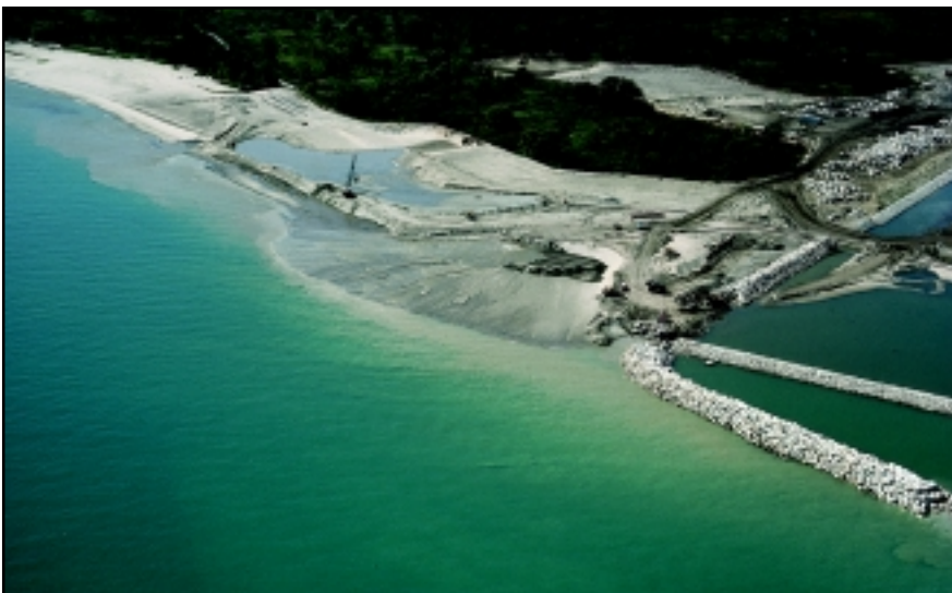
Figure 16: Dredged material from an Illinois marina construction project is being used for long-term beach nourishment. Credit: Illinois State Geological Survey
