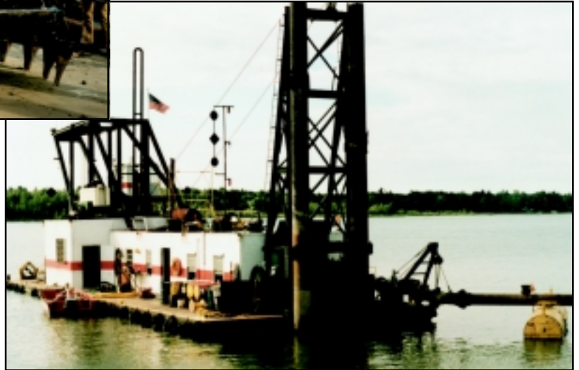
Figure 9: Hydraulic dredging with a pipeline.
