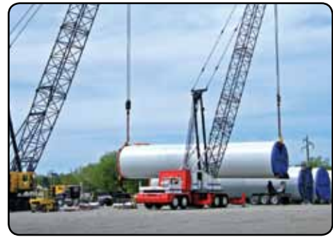
A wind turbine tower section is lowered onto a waiting truck at the port in Menominee, Mich., using the ship's cranes. The truck then moves to the staging area where tower sections are lifted by cranes and stored on the grounds. Photos © Dick Lund.
