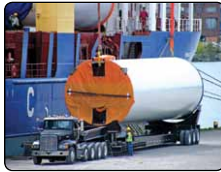
A wind turbine tower section is lowered onto a waiting truck at the port in Menominee, Mich., using the ship's cranes. The truck then moves to the staging area where tower sections are lifted by cranes and stored on the grounds. Photos © Dick Lund.
