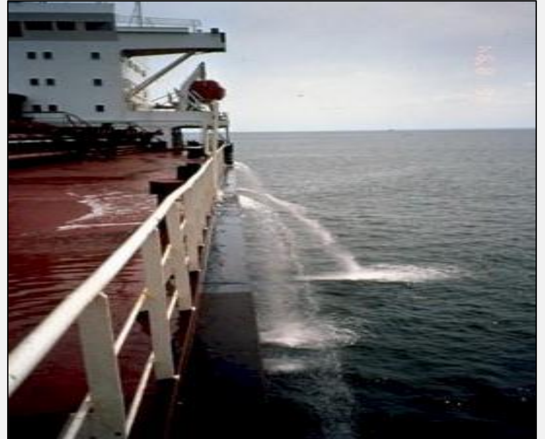
Water Overflowing from Deck Hatches and Ports During BWE; Photo courtesy of Smithsonian Environmental Research Center at: https://invasions.si.edu/nbic/managementpract.html
