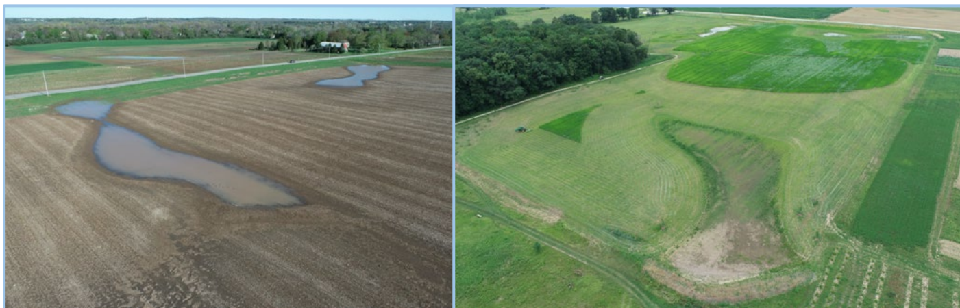
Ponding conditions which led to nutrient pollution downstream (left) were addressed through wetland construction and native prairie plantings on restored agricultural lands (right).
