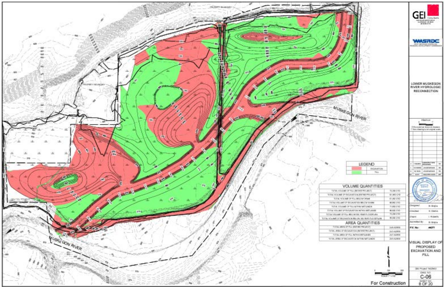
Appendix Figure 10. Proposed areas of fill (green) and excavation (pink) for the Lower Muskegon River hydrologic reconnection project.
