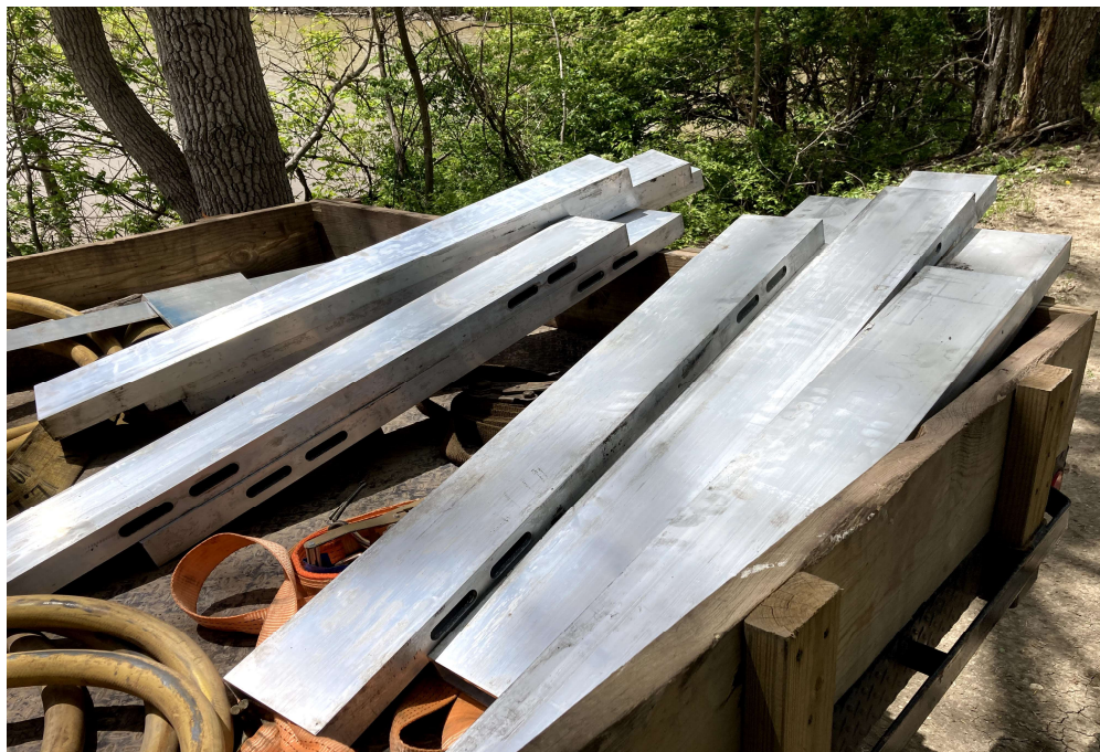
PHOTO 4: Overview of stop logs for the WCSs.
