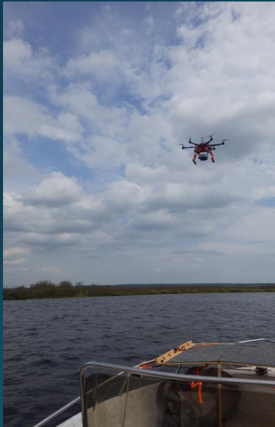
Boat-deployable platforms: the ~1 m diameter Bergen Hexacopter (left) and 350 mm DJI Phantom 15-20 minutes flight time, ~300m to 1 km radius, 15-30 ha
