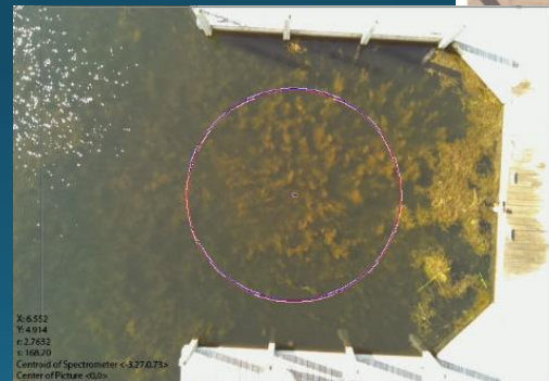
Reference photo overlaid with the footprint of the spectrometer at the water's surface
