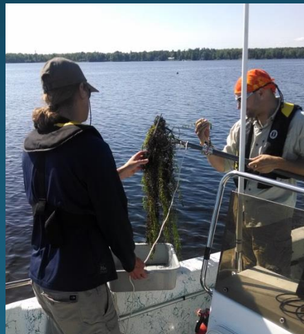
Twist rake sampling
